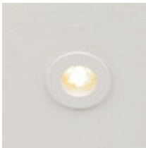
GIZMO DOWNLIGHT FIXED Comes with 1m cable Operated by external LED driver, max 700 mA / 2W, Vf = 3V
